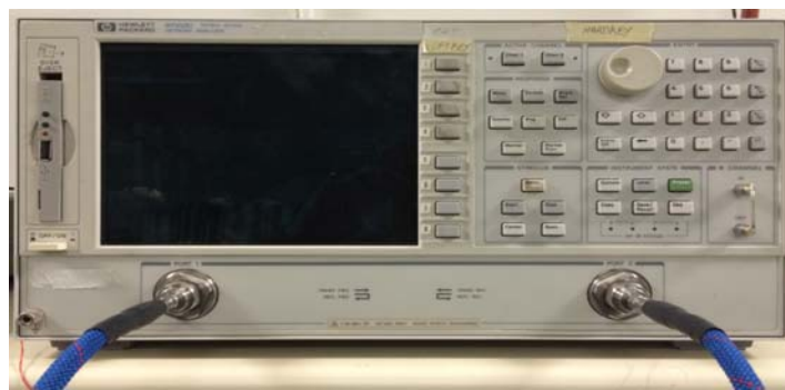
Figure 1.2: HP Model 8722D 40GHz Vector Network Analyzer.
