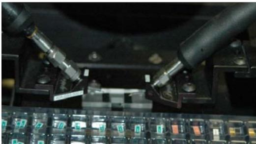
Figure 1 - measurement setup with G-S-G probes
