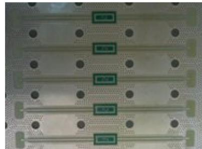
Figure 3 - Filters soldered in a wave-guide test board
