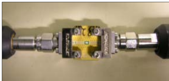
Fig 1: Assembled fixture with mounted coupon
